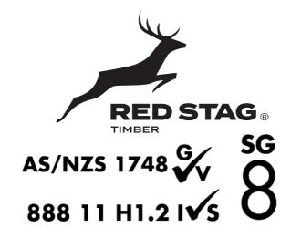
Mechanically stress graded SG timber intended for interior construction will have the grade and treatment identification at 1200mm centres along the board. Visually stress graded SG8 intended for exterior construction will have one grade and treatment identification at the end of the board.
