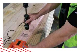
Measuring Moisture in radiata pine using a meter with long insulated prongs: Hammer 1/3 the way through the piece and at least 600mm from the end. Make sure batteries are fresh, meter is calibrated correctly and a correction is applied for species and treatment. For additional technical information about Red Stag Timber Products ask your merchant to arrange a training program with their Red Stag Timber professional.
