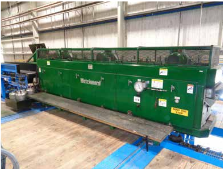
Metrigard Mechanical Stress Grader: 20 years more modern than any similar grader in New Zealand
