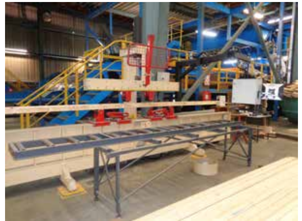
Proof Loader: One in 600 pieces is re-tested to confirm the mechanical testing process
