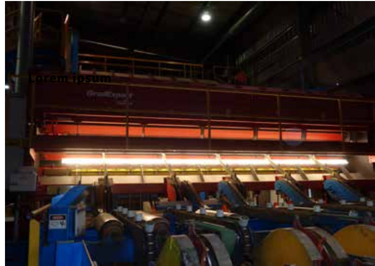
GradExpert: Optically grades for visual consistency and removes boards that fail to comply with this specification
